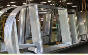
Winnie Drop features aluminum framing laminated with block foam insulation, true gel coat fiberglass exterior, and designer interior décor panels.
