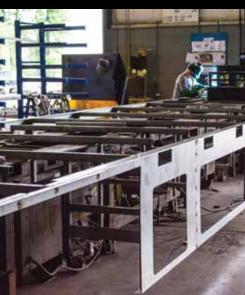
Structure built on a fixture table for optimum leveling and squareness. Laser cutting +/- 0.010. Bending within +/01 degree.
