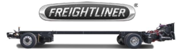
The Berkshire XL series utilizes the Freightliner XCR Raised Rail Chassis, Cummins ISL turbo diesel , 380 HP @2000RPM, 2200GOV RPM 1150 LB/FT @1400 RPM, and an Allison 3000MH 6-speed transmission
