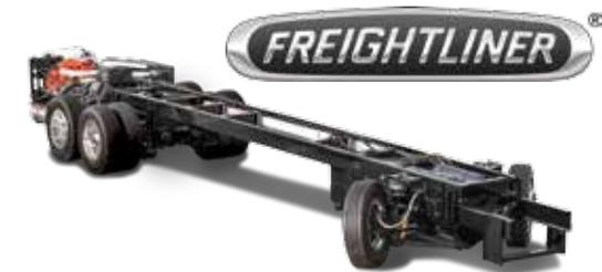
The Berkshire XLT series utilizes the Freightliner XCR Raised Rail Chassis, Cummins ISL 450HP @2100RPM, 2200GOV RPM, 1250 LB/FT @ 1400RPM and an Allison 3000MH 6-speed transmission
