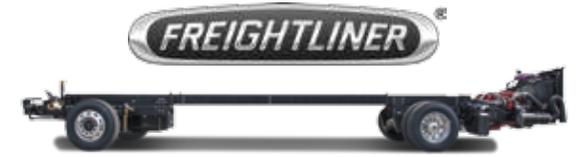
The Berkshire series utilizes the Freightliner XCR Raised Rail Chassis, Cummins ISB turbo diesel, 6.7 liter 340 HP at 2800 RPM, 700 ft. lbs. torque at 1600 RPM and an Allison MH-2500 6-Speed Automatic Transmission.
