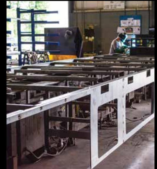
Structure built on a fixture table for optimum leveling and squareness. Laser cutting +/- 0.010. Bending within +/-01 degree.
