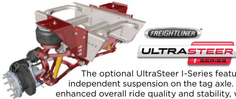
The optional UltraSteer I-Series features an independent suspension on the tag axle. This provides enhanced overall ride quality and stability, with comparable weight capacity and turning angle to the B-Series.\*
