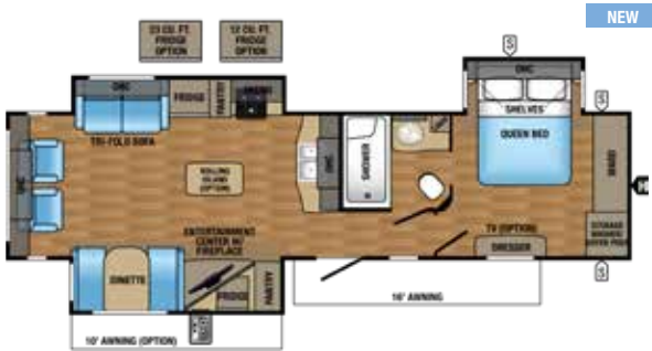
EAGLE TRAVEL TRAILER | 320RLTS OPTIONS: B, E Ext. Lgth: 38' 5" Ext. Ht: 141" Unloaded Wt (lbs.): 9,165 Sleeps: 4-6
