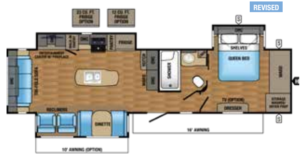
EAGLE TRAVEL TRAILER | 330RSTS OPTIONS: B, E, F Ext. Lgth: 39' 3" Ext. Ht: 137" Unloaded Wt (lbs.): 9,410 Sleeps: 4-6
