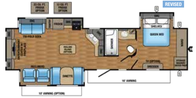
EAGLE TRAVEL TRAILER | 338RETS OPTIONS: B, C, E Ext. Lgth: 39' 3" Ext. Ht: 140" Unloaded Wt (lbs.): 9,130 Sleeps: 4-6
