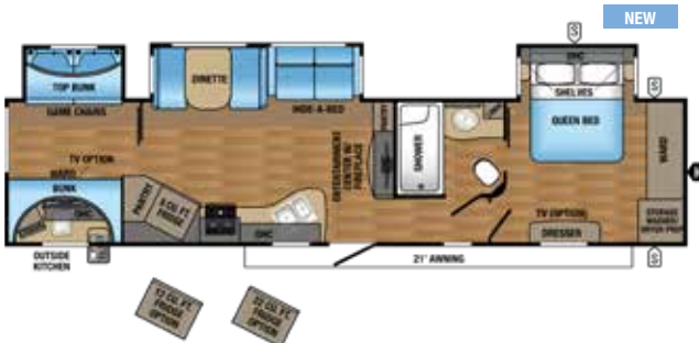
EAGLE TRAVEL TRAILER | 333BHOK OPTIONS: A, B, D, E Ext. Lgth: 41' 8" Ext. Ht: 142" Unloaded Wt (lbs.): 10,040 Sleeps: 8-10
