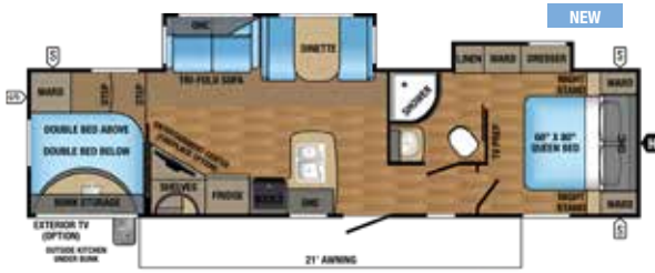
EAGLE HT TRAVEL TRAILER | 295DBOK OPTIONS: A, B Ext. Lgth: 37' 10" Ext. Ht: 138" Unloaded Wt (lbs.): 8,095 Sleeps: 6-10
