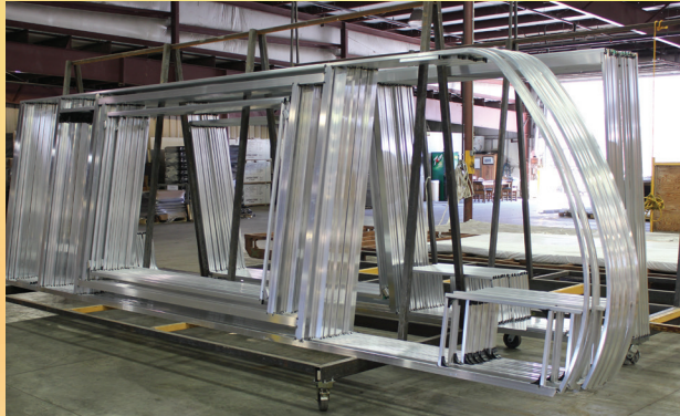
Minnie features aluminum framing laminated with block foam insulation, true gel coat fiberglass exterior, and designer interior décor panels.
