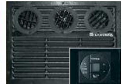
The Dometic Cool Cat 10,150 BTU heat pump is standard on Clipper hardside camping trailers.
