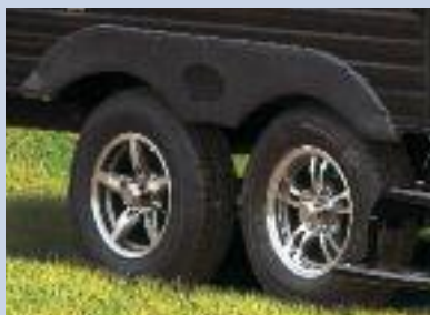
Tandem axles enhance stability
