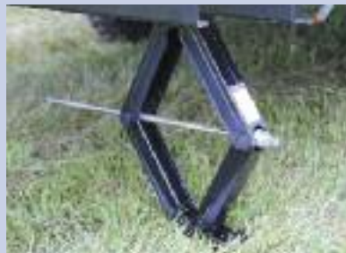
Four standard heavy duty stabilizing jacks
