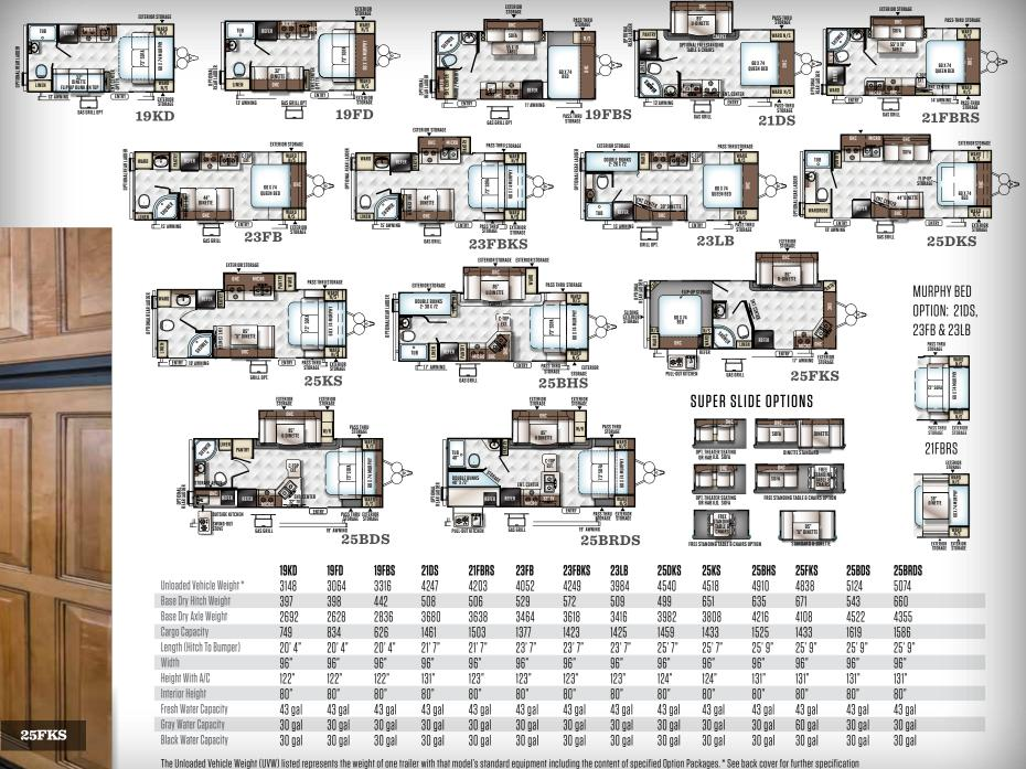
The Unloaded Vehicle Weight (UVW) listed represents the weight of one trailer with that model's standard equipment including the content of specified Option Packages.\* See back cover for further specification definitions.
