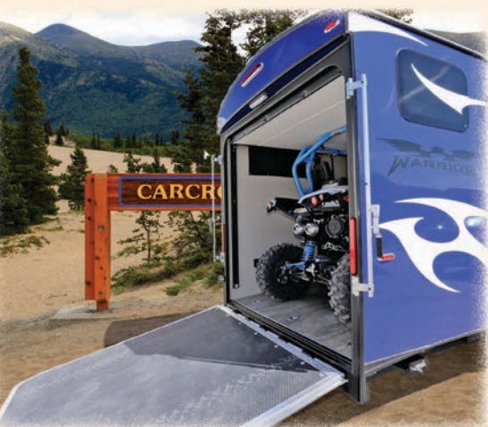
Beaver tail - extending the ramp angle for lowered vehicles - streets bikes and race cars
