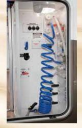
Docking Station includes outside shower, black tank flush, water bypass, 12V battery disconnect, selector switches, dump valves, water tank and city fills for centralized convenience.
