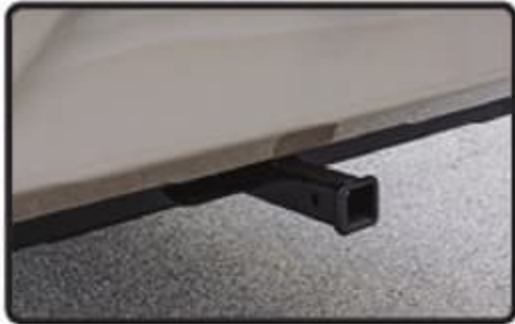
2" RECEIVER HITCH WITH 300 LB CAPACITY FOR YOUR ACCESSORIES
