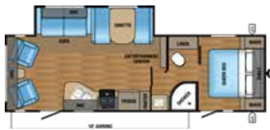
JAY FLIGHT SLX | 265RLSW Ext. Lgth: 30' 11" Ext. Ht: 133" Unloaded Wt (lbs.): 5,925 Sleeps: 4-6
