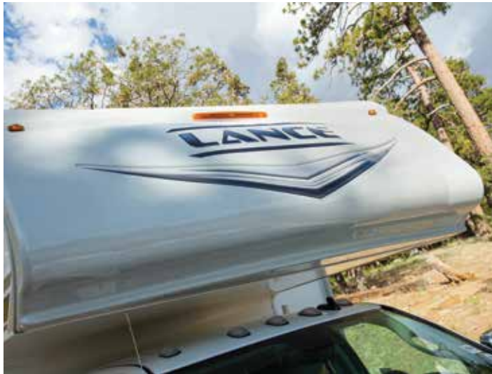
Aerodynamic TPO front nose cap protects your camper from debris and leaks while reducing drag and increasing fuel economy.
