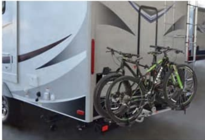
4" Rear Bumper & 1 1/4" Receiver Accommodates Bike Rack and Other Accessories (Load Limit of 130lbs.) (N/A 1475 & 1575)
