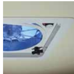
Fan-Tastic Vent allows for air circulation out of the trailer
