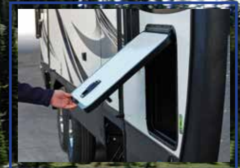
1" Thick Thermal Insulated Luggage Door Compartments
