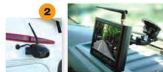
2 Wireless Rear-View camera/monitor maximizes safety
