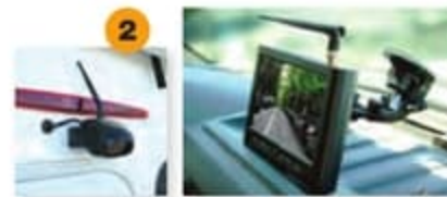
Wireless Rear-View camera/monitor maximizes safety
