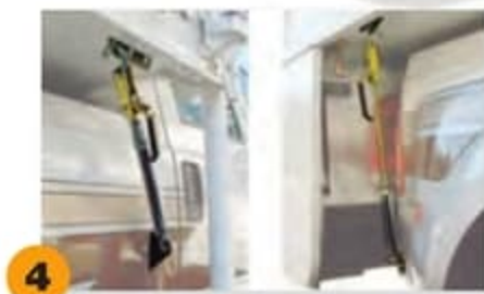
4 Qwik-Load Turnbuckle Upgrades make anchoring your camper a snap (Happijac® shown)
