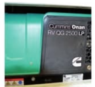
Propane Generator for charging your batteries, running the A/C or other 110 volt devices.
