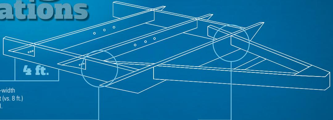
**Full-width outriggers:** We build on full-width outriggers that are spaced 4-6 feet apart (vs. 8 ft.) to better support the weight of the wall.
