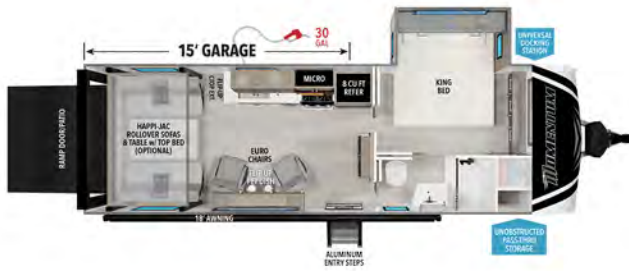
23G 15' GARAGE UVW' EMPTY HITCH' GVWR LENGTH' HEIGHT CAPACITY 7,669 1,242 13,000 28' 10" 12' 4" 90 74 39
