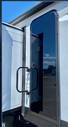
100% Safety Glass Entry Door with Dark Tint, Friction Hinge, Viewing Window and Shade Prep
