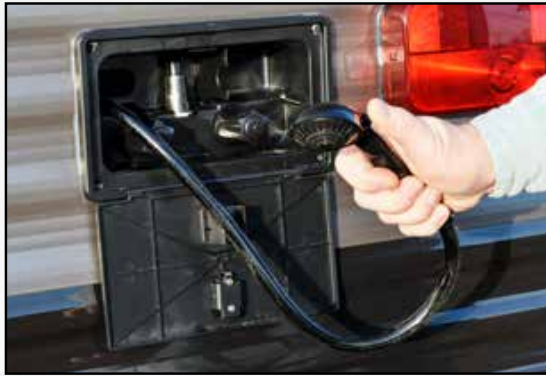
Outside Shower with hot and cold water.
