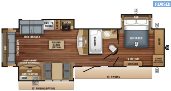
EAGLE TRAVEL TRAILER | 322RL0K OPTIONS: E, G Ext. Lgth: 38' 5" Ext. Ht: 146" Unloaded Wt. (lbs): 9,505 Sleeps: 4-6
