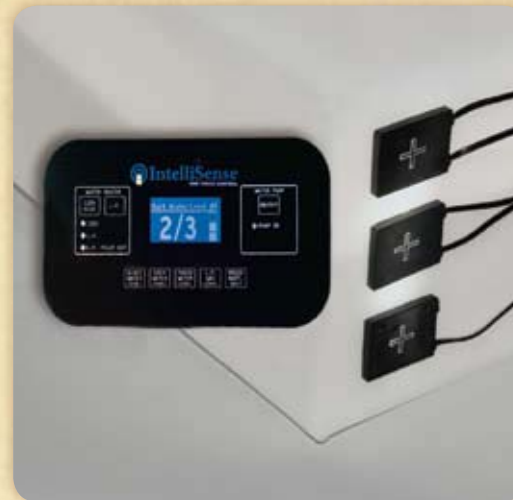
TRUELEVEL The TrueLevel holding-tank monitoring system uses sonar technology to read liquid levels from outside the tank. There are no probes to corrode or clog, just accurate readings time after time.
