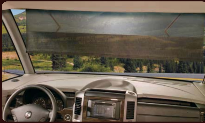
Sunvisor A powered sunvisor drops down at the touch of a button.
