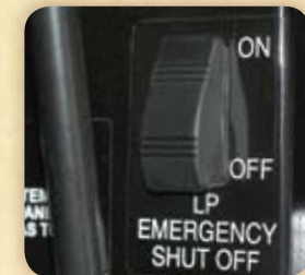
LP Tank Switch The LP tank has a remote switch for simple, safe operation.
