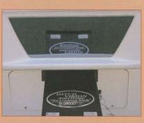
The innovative Hitch Vision™ mirror mounted on the center of the Montana front end makes it much easier to align the hitch pin of the fifth wheel to your truck.
