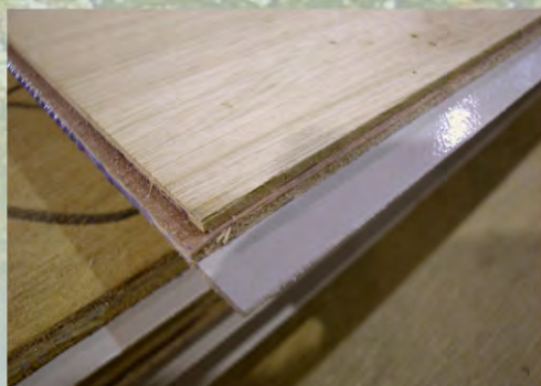
Multi Layered Laminated Fiberglass Wall
