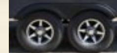
Optional aluminum wheels with Super Lube axles and ABS molded fender skirts
