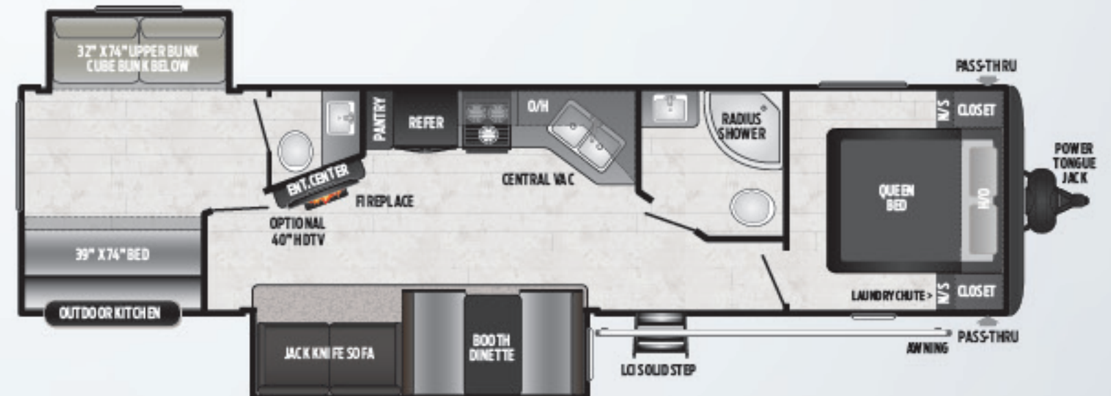
338LHS | TWO-SLIDE, PRIVATE BUNKROOM, BATH & A HALF, OUTDOOR KITCHEN Weight: 8061 LBS. | Length: 37' 11"
