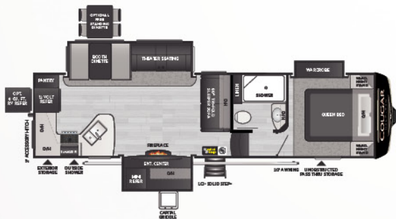
29RKS | WEIGHT 8958 | LENGTH 32' 9" HALF-TON FW • REAR KITCHEN, OPEN CONCEPT W/ OUTSIDE KITCHEN
