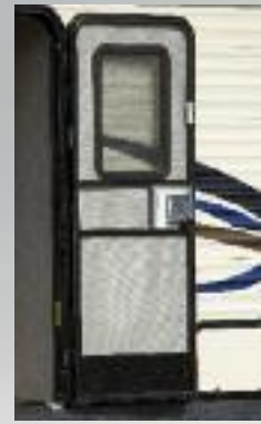
Friction hinge door with window and kick plate
