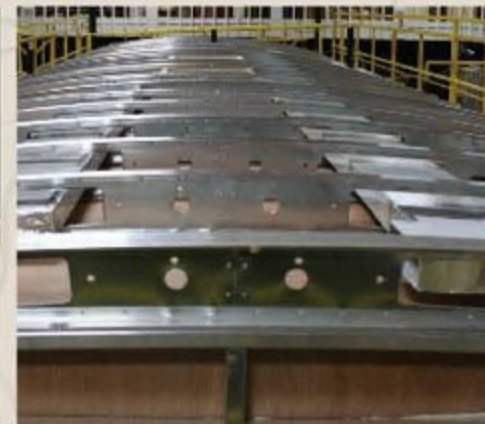
Walkable steel truss roof system
