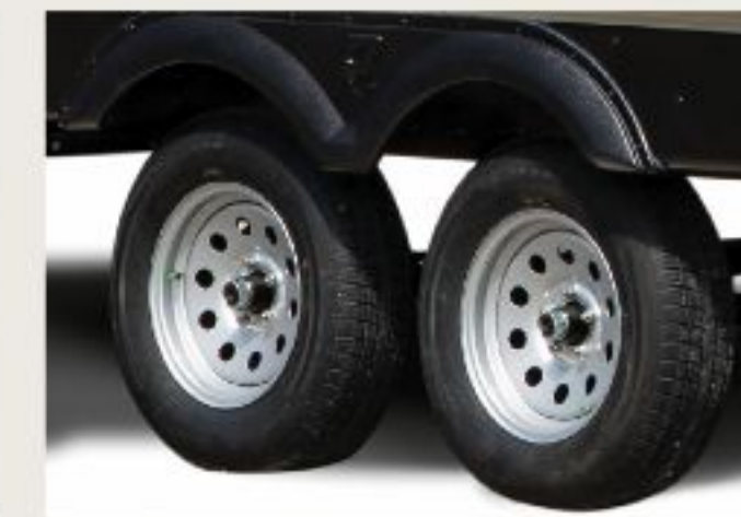
Grey steel wheel rims with Super Lube axles and ABS molded fender skirts
