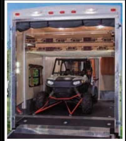
Garages include heavy duty tie-downs, anchored into an 8" x14" steel plate welded to the frame for secure travel.
