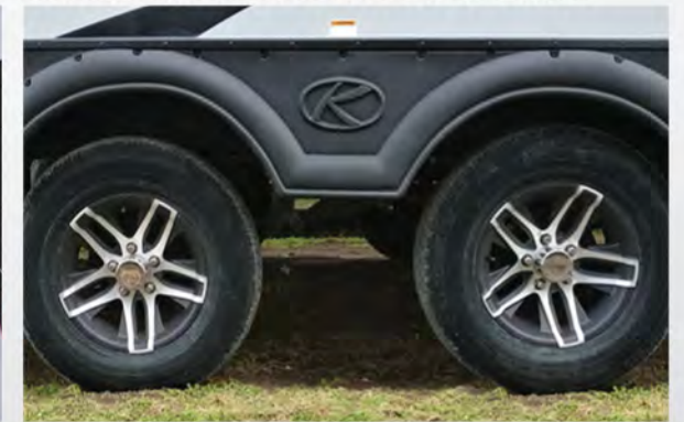
43" Wide Stance Dexter Axles with 15" Wheels
