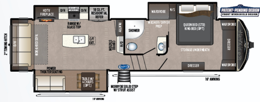
294/295RL | REAR LIVING ROOM, THREE SLIDES | Weight: 11035 LBS. | Length: 34' 0" RV REFRIGERATOR | RES. REFRIGERATOR
