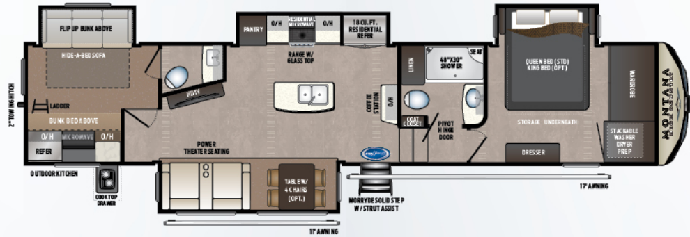
364/365BH | BUNKHOUSE W/ FULL BATH, HALF BATH, OUTSIDE KITCHEN | Weight: 12850 LBS. | Length: 40' 11" RV REFRIGERATOR | RES. REFRIGERATOR
