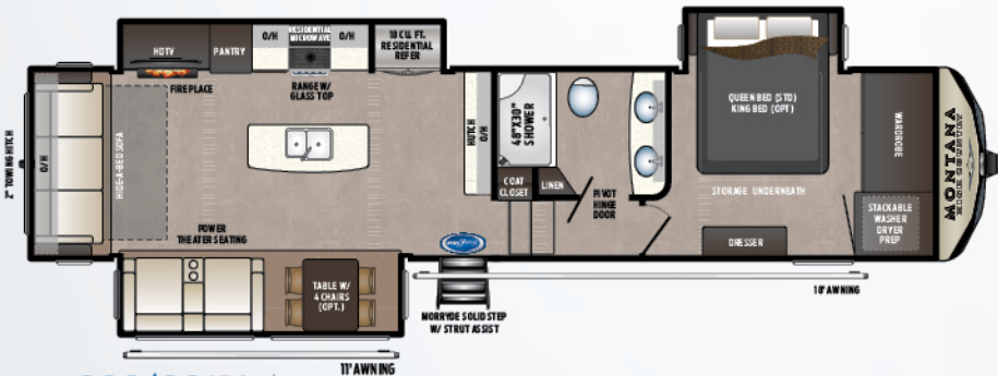
330/331RL | REAR LIVING ROOM, BATHROOM WITH DOUBLE VANITY | Weight: 11369 LBS. | Length: 37' 4" RV REFRIGERATOR | RES. REFRIGERATOR
