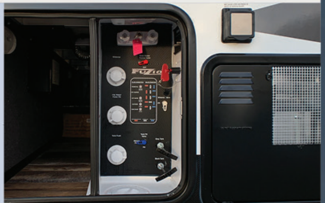
Exterior Convenience Center Complete with easy-to-read operation instructions for hook-ups, dry camping, black tank flush, winterizing, and more.
