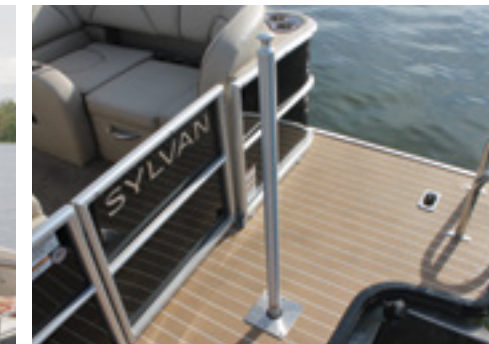
SKI PYLON Removable ski pylon that's bolted through the deck for maximum strength.
