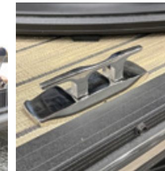
FOLD-UP CLEATS Through-bolted fold-up cleats fold up and down when needed.
