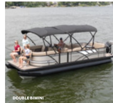
ENCLOSURE AND BIMINI OPTIONS Extend your season by getting away from the elements with an enclosure. They feature our Easy Match Tab System for quick assembly, sturdy round aluminum tubing and stainless features for strength, quick release for ease of use, and solution-dyed polyester Vista canvas for lasting color without bleeding.
