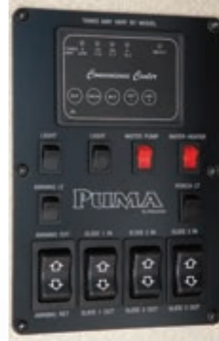
Convenience Center shows battery/tank capacities. Controls slides, awning, interior/porch lights, water pump/heater
