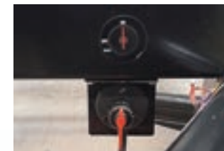
Seafo battery isolator switch prevents power drain. Operates by removable key
