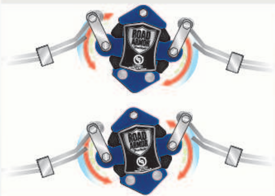
EXCLUSIVE Road Armor™ Suspension Equalizes axle load to dampen shock and vibration.
