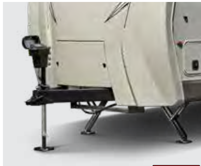
TRAVEL TRAILER ELECTRIC AUTO-LEVELING SYSTEM (BAL 5.3)
