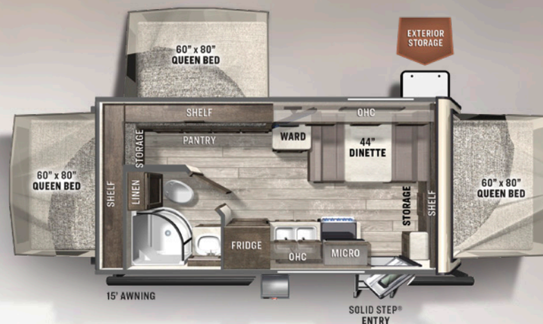
183 EXPANDABLE U/V: 4299 HITCH: 480 AXLE: 3781 LENGTH: 21'2" OPEN LENGTH: 25'7" ROO CCC: 1461 WIDTH: 8' HEIGHT: 10'6" FRESH: 54 gal GRAY: 30 gal BLACK: 30 gal
