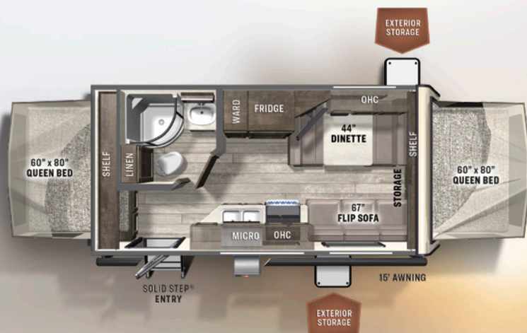
19 EXPANDABLE U/V: 4137 HITCH: 448 AXLE: 3651 LENGTH: 21'2" OPEN LENGTH: 25'7" ROO CCC: 1591 WIDTH: 8' HEIGHT: 10'6" FRESH: 54 gal GRAY: 30 gal BLACK: 30 gal
