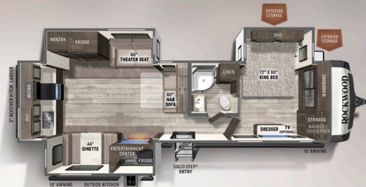
8332SB REAR KITCHEN SIGNATURE UVW: 9444 HITCH: 1130 AXLE: 8255 CCC: 1686 LENGTH: 36'8" WIDTH: 8' HEIGHT: 11'7" FRESH: 54 gal GRAY: 110 gal BLACK: 50 gal
