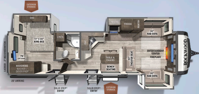
8324SB FRONT LIVING SIGNATURE UVW: 9254 HITCH: 1115 AXLE: 8080 CCC: 1861 LENGTH: 36'8" WIDTH: 8' HEIGHT: 11'7" FRESH: 54 gal GRAY: 120 gal BLACK: 50 gal
