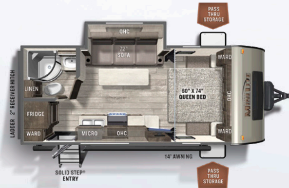
2109S REAR LIVING UVW: 4171 HITCH: 412 AXLE: 3700 CCC: 1521 LENGTH: 22' 4" MINI LITE WIDTH: 8' HEIGHT: 10' 3" FRESH: 54 gal GRAY: 30 gal BLACK: 30 gal
