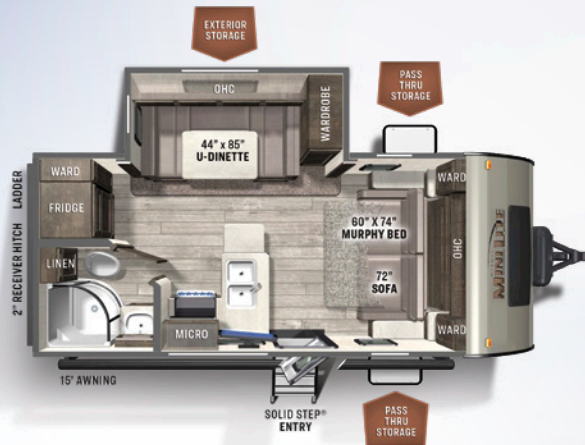
2104S MURPHY BED UVW: 4841 HITCH: 614 AXLE: 4168 CCC: 1933 LENGTH: 22' 4" MINI LITE WIDTH: 8' HEIGHT: 10' 11" FRESH: 54 gal GRAY: 30 gal BLACK: 30 gal
