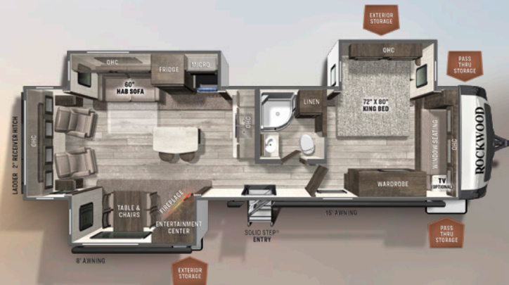
8329SB REAR KITCHEN SIGNATURE UVW: 8839 HITCH: 1130 AXLE: 7650 CCC: 2291 LENGTH: 36'8" WIDTH: 8' HEIGHT: 11'7" FRESH: 54 gal GRAY: 80 gal BLACK: 50 gal
