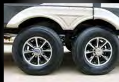
Contemporary aluminum rims with E-rated radial tires. Most SIERRA's feature 7000 Lb. axles.
