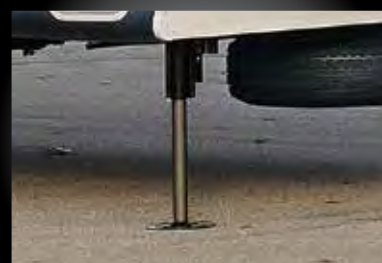
Wide stance hydraulic landing gear.
