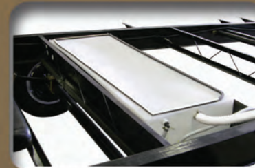
Heated and Enclosed Fresh Water Tank
