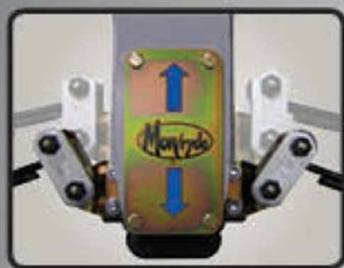
EXCLUSIVE MOR/RYDE 4100 SUSPENSION SYSTEM W/ WET BOLTS
