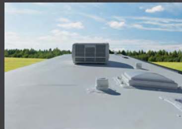
Seamless Roofing Membrane with Heat Reflectivity
