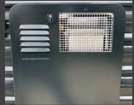
6 Gallon Gas/Electric DSI Water Heater
