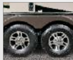
Premium Goodyear® E-rated tires are standard on all models with 8-lug, easy lube axles and aluminum alloy wheels. (G-rated option available)
