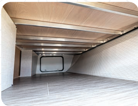
WELDED ALUMINUM BED FRAMING (16/19 SERIES ONLY)
