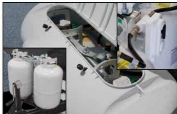
30# LP Bottles and cover with easy access to auto changeover valve.
