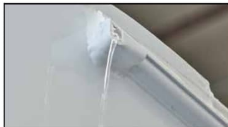
Innovative RAIN GUTTERS channel rain water away from your RV helping to reduce unsightly stains on sidewalls.
