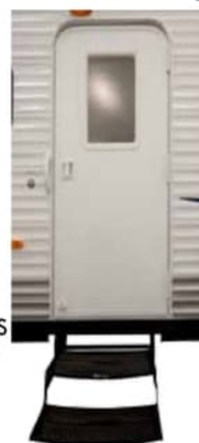
Radius door corners are stronger, last longer and don't tear awnings.
