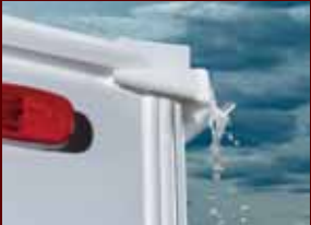
Another KZ standard – newly designed drip rails and spouts keep the water flowing away from the sidewalls.
