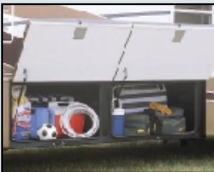
In every Intruder 2000 you'll find an amazing amount of storage space. Consider our underfloor, exterior-access storage compartments. Most of them have 22"-high openings outside the main rails and 12" pass-through areas. All these compartments are made of rugged rotocast polyethylene
