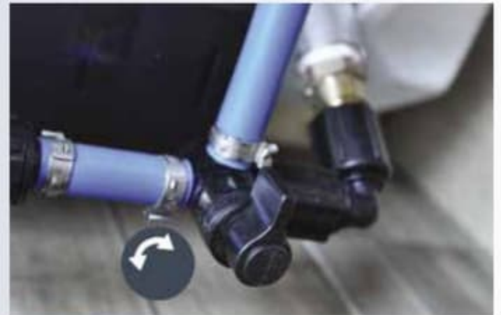
Water heater bypass & winterizing valves make draining the system for winter storage a breeze.
